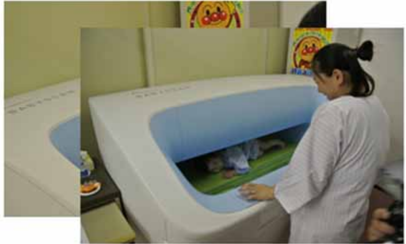
Whole Body Counter (Babyscan) used today Detection limit: 50 Bq/body
